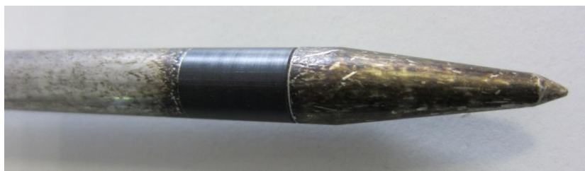
Soiled probe -> wrong measuring!
