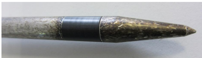
Soiled probe -> wrong measuring!
