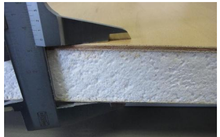
Sandwich Sperrholz – Isolation - Aluminium
