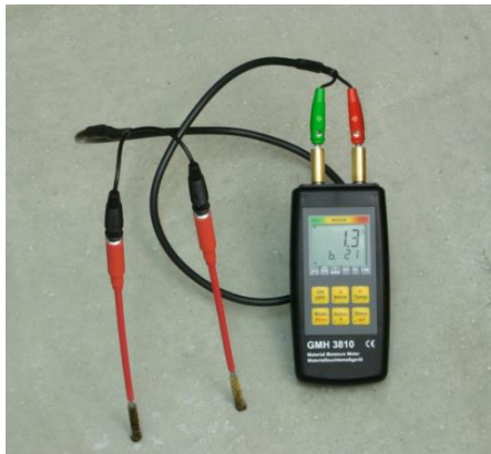
Measuring with brush probe GBSL91
