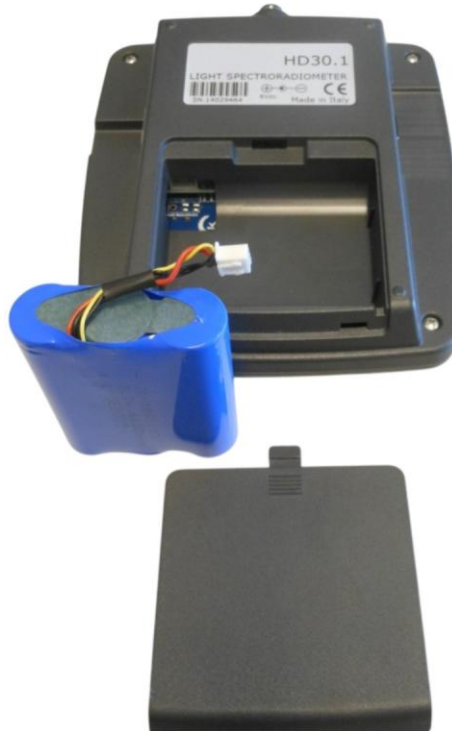
Fig. 2.2: battery removed from compartment
