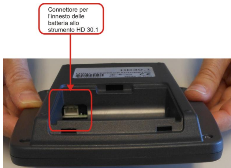
Fig. 2.3: instrument battery connector
