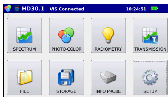
Fig. 3.2: start-up screen with HD30.S1 probe connected
