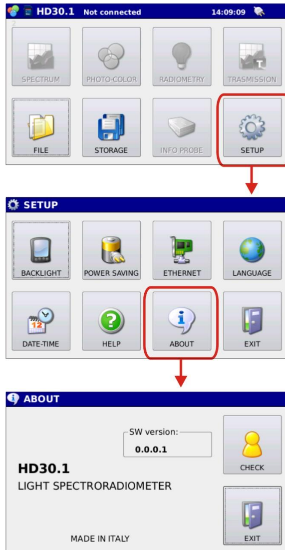
Fig. 5.1: sequence to be followed for software update
