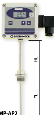
GTMU-MP-AP2 for high temperatures Standard type: G = ½", HL = 100 mm, FL = 100 mm, D = 6 mm
